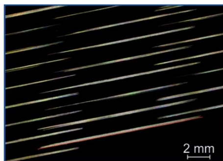
Figure 11. Sample texture manufactured with the grinding wheel with defined pattern
